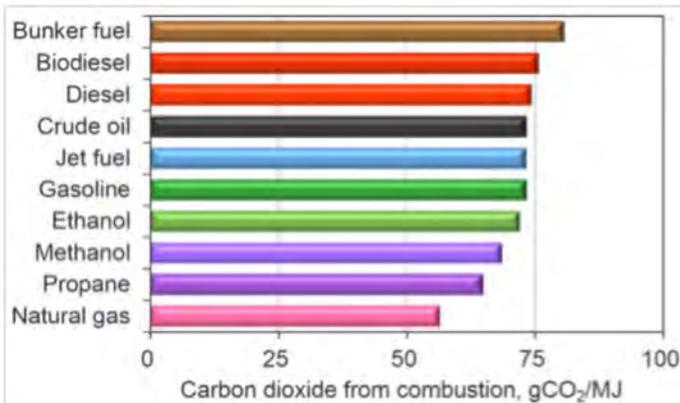
**Figure 1. CO2 emissions per unit of energy for various fuels.**
